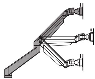
You can change the strength of the gas lift with an allen key on the rear of the monitor arm. This allows you to adjust the monitor arm to the weight of your monitor.
